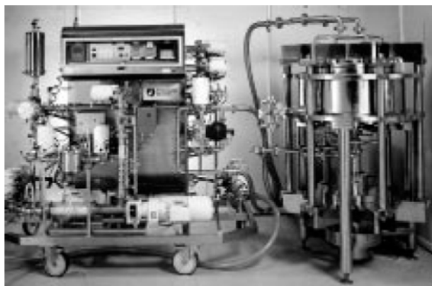
Fig. 9. Industrial scale chromatography system designed for use with 15 \mu\text{m} or 30 \mu\text{m} Source TM PS/DVB media. The volume of the 80 cm diameter stainless steel column is 50 l. (Courtesy: Amersham Pharmacia Biotech).
