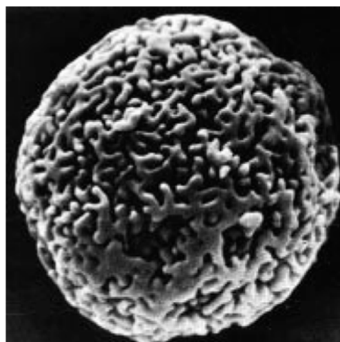
Fig. 2. LiChrospher Si 4000, dp 10 µm (Merck AG, Darmstadt, Germany).
